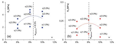
**Figure 4** Mix design of  $FF_wCC_w$  mixture:  $R_c$  (a) and  $R_{it}$  (b) vs. c and w
