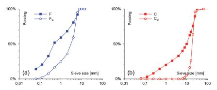
Figure 2 Gradations of selected stockpiles: a) fine aggregates F and F<sub>w</sub>, b) coarse aggregates C and C<sub>w</sub>
