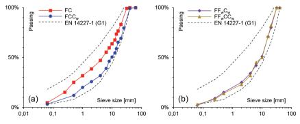
Figure 3 Final gradations of mixtures:a) FC,  $FCC_w$ , b) FFwCw,  $FF_wCC_w$
