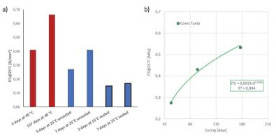
Figure 2 Evolutions of ITS values during the curing period of: a) sepcimens, b) cores
