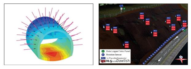
Figure 4 Tunnel Deformation Model
