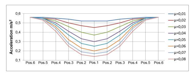
Figure 3 Resulting acceleration in relation to mass ratio and damper position
