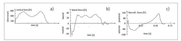
Figure 1 Walking force in (a) vertical, (b) lateral and (c) longitudinal direction [3]
