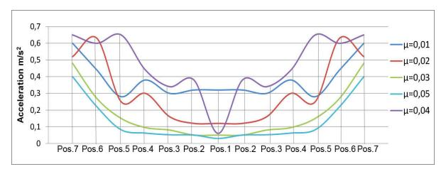
Figure 4 Graphical representation of the mass ratio and damper position
