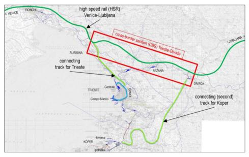
Figure 2 Connection lines to the Mediterranean Corridor in the area of Trieste and Koper.
