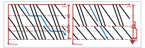
**Figure 2** On the left: typical timetable structure on major Budapest suburban lines. The blue path is the fastest possible freight path. On the right: increasing capacity by new tracks for faster trains in the inner zone. The blue path shows that the freight train is faster, even though the frequency of suburban trains is doubled
