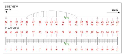
Figure 6 Positions of accelerometers and RTS measuring points
