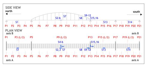
Figure 5 Measuring points of static vertical displacements (red) and measuring points for strain measuring (blue)
