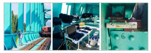
Figure 4 Vertical displacement measurement (left), data acquisition system (middle) and strain measurement sensor (right) on bridge "Sava"
