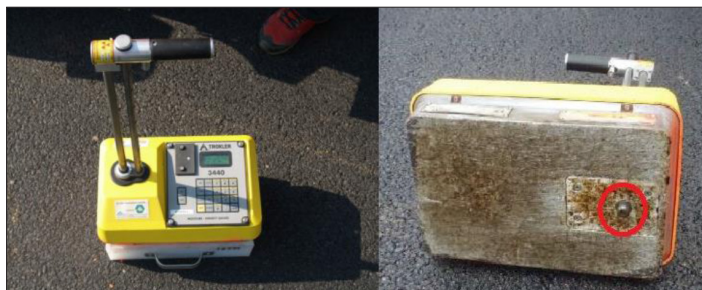
Figure 1 Troxler 3440 on the reference block [10]
