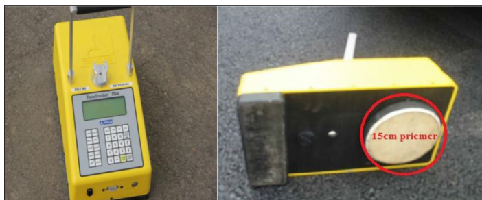
Figure 2 Troxler 2701-B, PaveTrackerTM [10]
