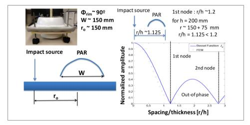
Figure 3 Optimal parameters for the PAR
