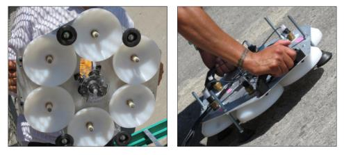
Figure 4 Hexagonal air-coupled acoustic array: parabolic reflectors with microphones and an impact source in the center (left), and application of the array in evaluation of a concrete dam
