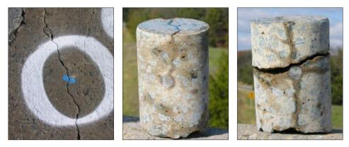
Figure 1 Vertical crack on the surface of a bridge deck (left), a core with a vertical crack (middle), and a core with a vertical crack and delamination (right)
