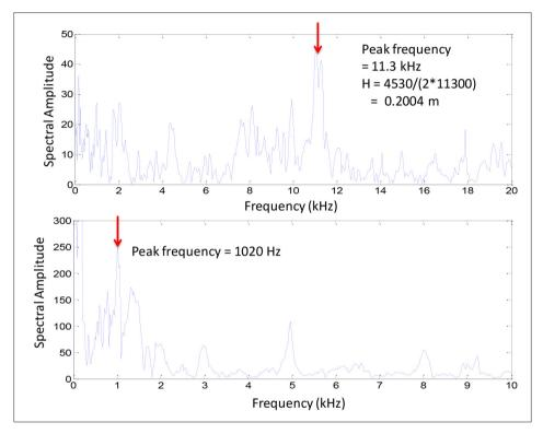
Figure 6 Frequency spectrum from IE survey at a location with no delamination (top), and a location with shallow delamination (bottom)
