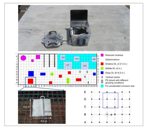
Figure 5 Hexagonal air-coupled acoustic array on the validation bridge (top), schematic of embedded defects and deterioration in the bridge (middle), and the delamination evaluated (bottom)
