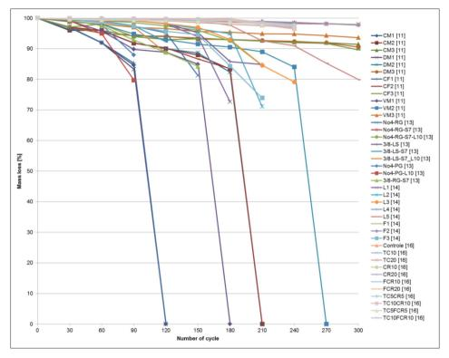
Figure 4 Frost resistance of pervious concrete at 28 days
