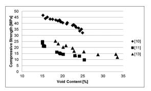
Figure 1 Plot of compressive strength as a function of void content
