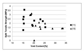
Figure 2 Plot of splitting tensile strength as a function of void content
