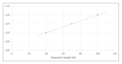
Figure 8 Proportion between internal forces obtained on loaded and unloaded conditions in function of the expansion length of the bridge
