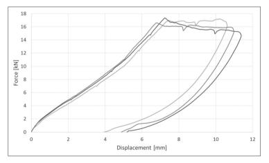
Figure 2 Force-displacement diagram of KS fastening
