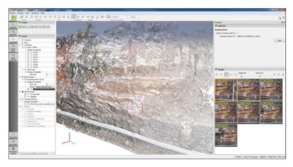
Figure 7 Point cloud generated by Pix4Dmapper Pro from photos taken from air
