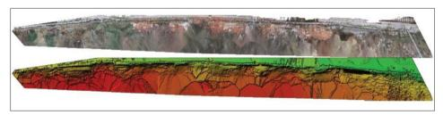
Figure 6 Ortophoto map and Digital Surface Model (DSM) generated by Pix4Dmapper Pro from photos taken from air
