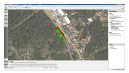
Figure 5 Screen shot of Pix4D mapper Pro with positions where images were taken
