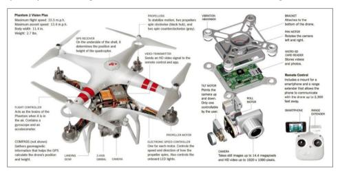
Figure 2 Parts of DII Phantom 2 Vison+
