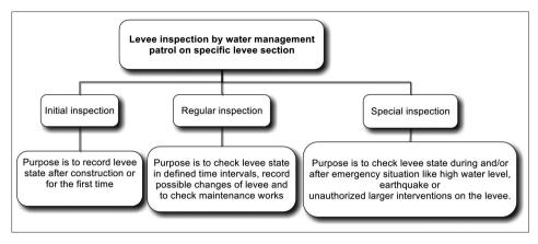
Figure 3 Types of levee inspection by water management patrol
