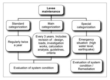
Figure 2 Guidelines for frequency of levee assessment [1]
