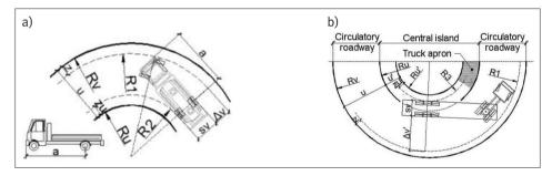
Figure 1 Determination of the circulatory roadway and truck apron width [4]
