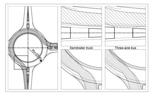
Figure 4 Semitrailer truck and three-axle bus movement trajectories
