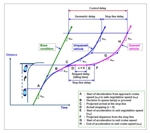
Figure 1 Definition of control delay, geometric delay, stop – line delay and stopped delay (Source: Sidra Intersection – User Guide) [3]
