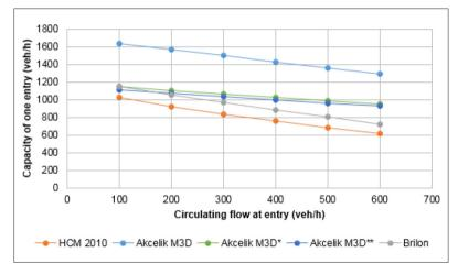
Figure 2 Comparison of roundabout capacity for different metodologies
