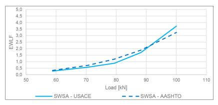
Figure 2 Equivalent wheel load factors in overload axles – Single Wheel Single-Axle
