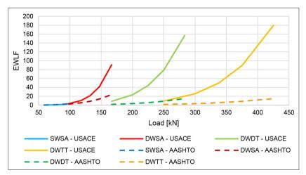
Figure 1 Equivalent wheel load factors in overload axles
