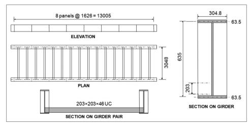
Figure 2 Example U-frame bridge deck
