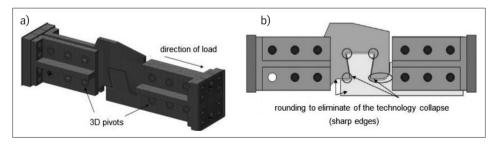
Figure 8 FE models mapping two different shapes of the lock connectors (as in the experimental tests): a) initial hook-shape lock, b) modiffied dovetail joint without sharp edges
