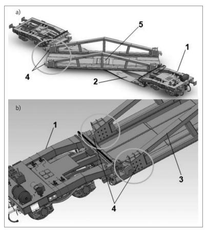
Figure 1 Prototype version of the wagon with :a) the open loading platform, b) the closed loading platform with the view of lock components: 1 – over-bogie part of the wagon, 2 – the lowered fixed frame of wagon, 3 – the side of the moving loading platform, 4 – hook shape locks with suppert area, 5 – central node of the rotatable platform
