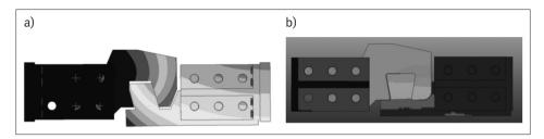
Figure 9 Displacement maps for: a) initial shape of the hook-lock connector, b) modiffied dovetail joint
