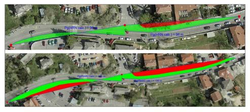
Figure 2 Sight triangle visualisations for left turn from minor road considering calculated sight distance using Croatian standard (upper scheme) and PIARC's RSM (lower scheme)
