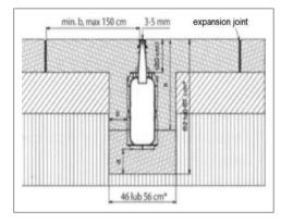
Figure 5 Keyway slot heavy- type version of male
