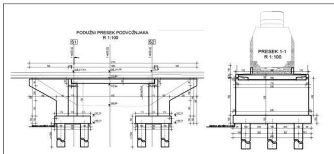
Figure 3 Underpass with length L=21.50m at km 1+485.02 [1]
