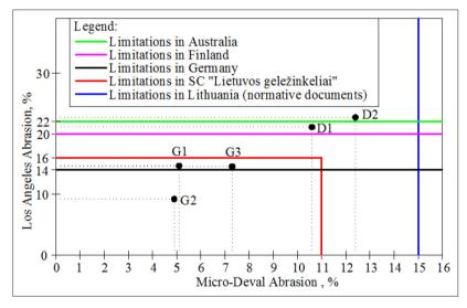
Figure 1 Determination results of particles resistance to wear and fragmentation and maximum permissible values of these parameters in Lithuania and abroad.
