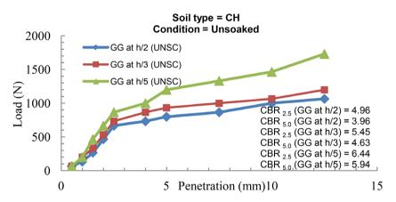
Figure 3 Load v/s penetration curve for SIL of GG at different position (UNSC)
