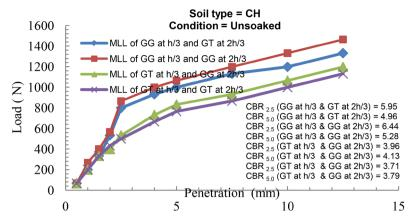
Figure 8 Load v/s penetrations for MLL for various positions of GT and GG
