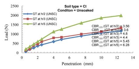
Figure 2 Load v/s penetration curve for SIL of GT at different position (UNSC)
