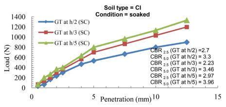
Figure 1 Load v/s penetration curve for SIL of GT at different position (SC)
