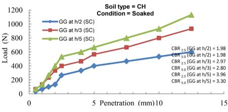
Figure 4 Load v/s penetration curve for SIL of GG at different position (SC)
