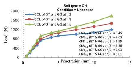
Figure 6 Load v/s penetration curve for COL for various positions of GG and GT
