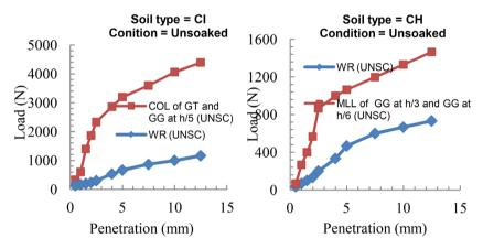
Figure 9 Load v/s penetration curve for comparison of WR with COL and WR with MLL for GT and GG at h/5 (UNSC)
