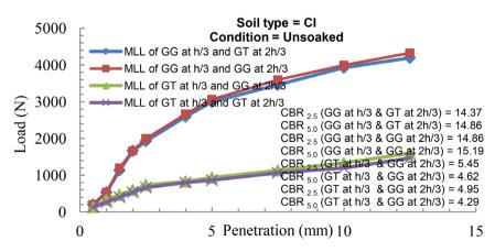
Figure 7 Load v/s penetration curve for MLL for various positions of GT and GG
