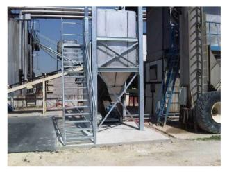
Figure 2 Automated feeding of the additive (Plant CIFA Mitry-Mory, France)
