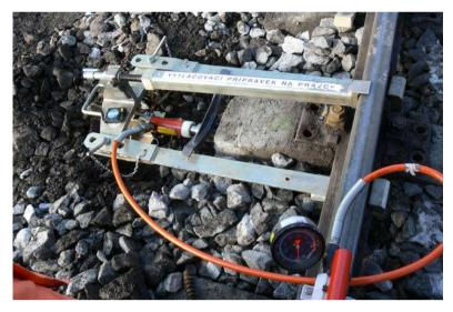
Figure 7 Extruder device
