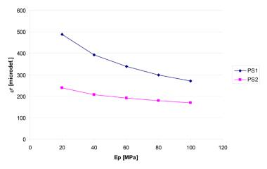
Figure 1 Horizontal tensile strain variation at the base of bituminous layers.
