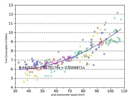
Figure 5 Fuel consumptions variations for the whole anemometer speed range (planned vehicle speeds of 50, 75 and 100 km/h ;  $4^{th}$  gear ratio)
