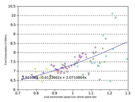
Figure 6 Influence of airflow speed over vehicle speed ratio (A/V ratio) on fuel consumptions (vehicle speed of 75 km/h; 4<sup>th</sup> gear ratio)
