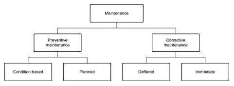
Figure 2 Types of maintenance of railway track [3]
