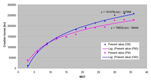
Figure 3 Comparison of corrective and preventive maintenance costs (present values) based on cumulative traffic load for standard kilometer IIb (7,5 kn = 1,0 EUR)
