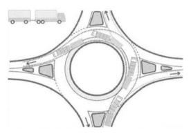
Figure 5 Offtracking control at roundabouts [8]
