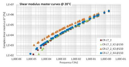
Figure 2 Complex shear modulus master curve for CRmBs with different catalysts
