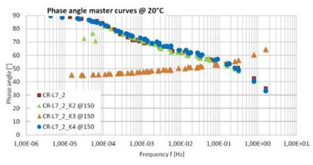
Figure 3 Phase angle master curve for CRmBs with different catalysts
