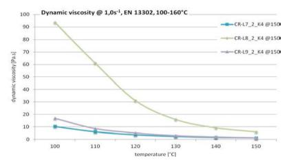
Figure 4 Flow (viscosity) curves for CRmBs with pulverized rubber of different grading
