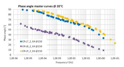
Figure 6 Phase angle master curve for CRmBs with pulverized rubber of different grading
