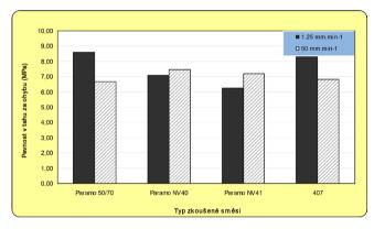
Figure 2 Results of flexural strength test, set I
