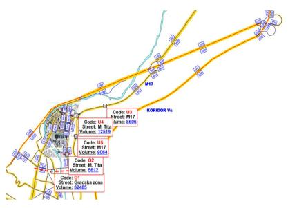
Figure 6 Traffic volume Scenario III – with the Corridor Vc and the South Bypass
