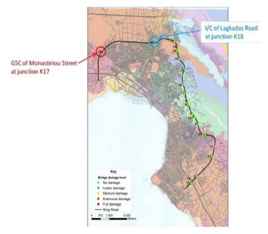
Figure 2 Visual representation of locations and bridge damage level on the Inner Ring Road Using the BDI and LDI indices:
