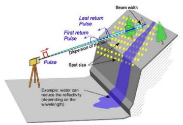
Figure 2 Principles of laser scanning for terrestrial lasser scanner (TLS) [7]
