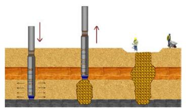
Figure 3 Vibro-stone columns (vibro-replacement) technique
