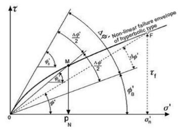
Figure 1 Non-linear failure envelope of hyperbolic type and its parameters.
