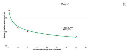
Figure 4 The ratio of compaction energy and the altitude of asphalt specimens
