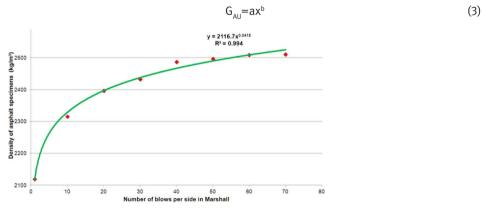
Figure 5 The ratio of variable energy and densities of asphalt specimens
