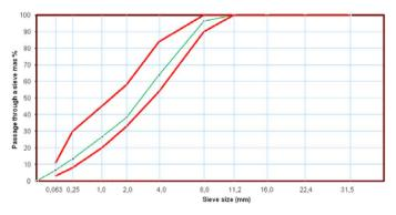
Figure 1 Gradation of the designed asphalt mixture
