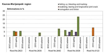
Figure 6 Results of the visual assessment of the trial sections with double Otta seal
