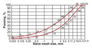
Figure 2 Gradation curves for the double Otta seal aggregate
