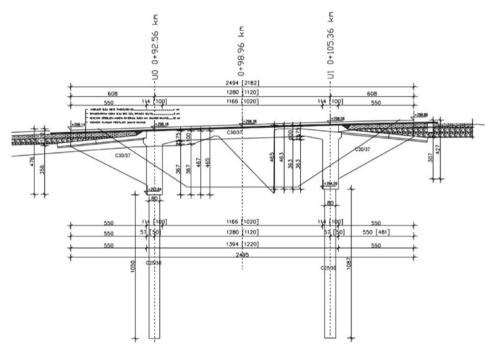
Figure 3 "Anđeli" viaduct longitudinal profile
