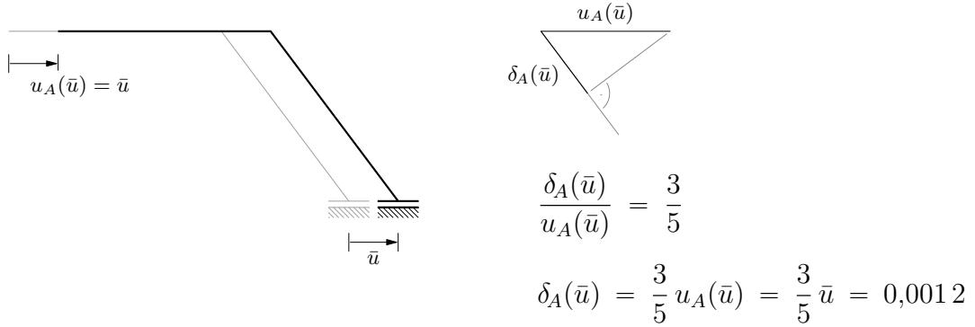
$$\delta_A = \delta_A(M) + \delta_A(\bar{u}) = 0,000\,738\,477 + 0,001\,2 = 0,001\,938\,48 \text{ m} = 1,94 \text{ mm}$$
