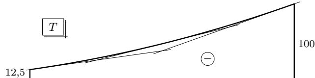
$$\begin{aligned} & \text{Diagram showing internal forces } Q_1(x), Q_2(x), q(x) \text{ and moments } T(x), M(x) \text{ at position } x. \\ & q(x) = q_1 + \frac{q_2 - q_1}{\ell} x = 10 + \frac{15}{5} x = 10 + 3 \cdot x \\ & Q_1(x) = \frac{1}{2} \cdot 10 \cdot x = 5 \cdot x \\ & Q_2(x) = \frac{1}{2} \cdot (10 + 3 \cdot x) \cdot x = 5 \cdot x + \frac{3}{2} \cdot x^2 \end{aligned}$$
