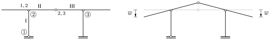
$$\delta_{1,0} = \bar{\delta}_{1,0} = -\bar{w} \quad \dots \text{prema planu pomak}\bar{a}$$
