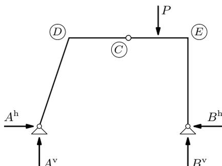
$$\sum_{\widehat{AB}} M_{/B} = 0 : \quad -5 \cdot A^v + 1 \cdot P = 0 \quad \Rightarrow \quad A^v = \frac{P}{5} = 20 \text{ kN}$$
