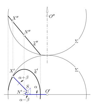
Figure 5: *The top view of a spherical trochoid is a planar trochoid of order three. It can be generated by an open three-bar mechanism.*
