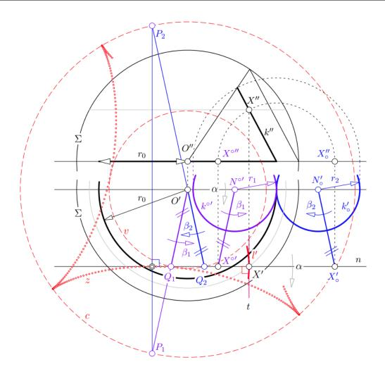
Figure 11: The top-view l' of a spherical trochoid is the involute of a hypocycloid z. The two different flips of k's plane are displayed in different colors (blue = to the outside, violet = to the inside).
