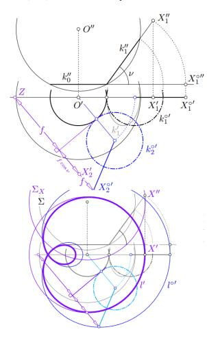
Figure 8: Top: The similarity factor between l' and  $l^{\circ'}$  depends on the inclination of the rolling circle's plane. Bottom: The fixed and moving polhodes are congruent and the top-view shows a symmetric rolling. Therefore, l' is a Pascal limaçon, as is  $l^{\circ'}$ .
