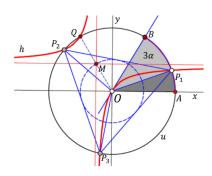
Figure 3: Angle trisection as the intersection of the unit circle u with the "Bolyai-hyperbola" h.
