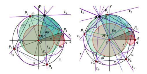
Figure 11: Angle 4-section and 5-section with help of epicycloids.
