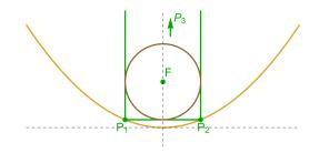
Figure 3: Construction used to derive r/f in Proposition 1. Side  $P_1P_2$  of the Poncelet triangle is perpendicular to the axis while the other two sides are parallel to it, i.e., vertex  $P_3$  lies on the line at infinity.
