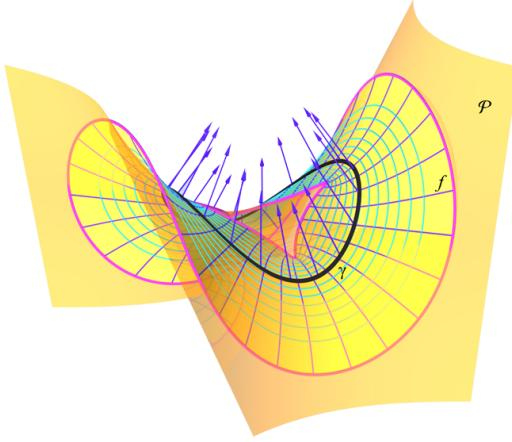
Figure 9: *The minimal surface (41) on the scroll  $(\gamma, v)$ . The curve  $\gamma$  is a curve along which the Gaussian curvature on the hyperbolic paraboloid  $P$  is constant.*
