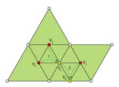
Figure 5: An example for propagation of inflexibility: 1. the two inflexible vertices  $v_1$  and  $v_2$  will cause  $v_a$  to become inflexible. 2.  $v_a$  together with the already existing inflexible vertex  $v_3$  induce a further inflexible point  $v_b$ .
