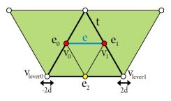
Figure 7: In order to keep the distance between two inflexible vertices  $v_0$  and  $v_1$  constant, their displacements have to be applied twice to the corresponding vertices  $v_{lever0}$  and  $v_{lever1}$  instead to  $v_0$  and  $v_1$ .
