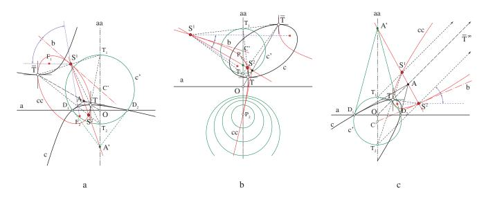
Figure 7: In figure a, conic c is a hyperbola,  $D_1$ ,  $D_2$  are real points and cc is an ellipse that cuts as at imaginary points. In figure b, conic c is an ellipse,  $D_1$ ,  $D_2$  are imaginary points and cc is a hyperbola that cuts as at Poncelet's points of  $\mathcal{P}(c,a)$ . In figure c, conic c is a parabola,  $D_1$ ,  $D_2$  are real points and cc is a parabola that cuts the line as at the pair of imaginary points.
