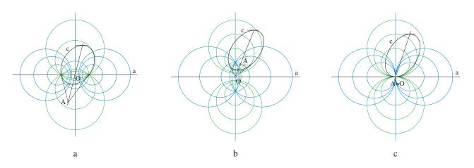
Figure 4: A is the pole of a with respect to c, and O is the midpoint of the orthogonal pencils of circles. The conic c and the line a with real and different, imaginary or coinciding intersection points, together with the corresponding Apollonian circles, are shown in figures a, b and c, respectively.
