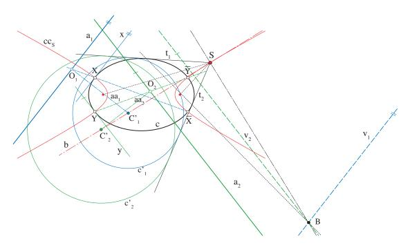
Figure 9: Circles  $c'_1$  and  $c'_2$  are the images of c under the central collineations with the center S and axes  $a_1$  and  $a_2$  with vanishing lines  $v_1$  and  $v_2$ , respectively. For any other central collineation with center S that transforms c into a circle, the vanishing line is either  $v_1$  or  $v_2$ .
