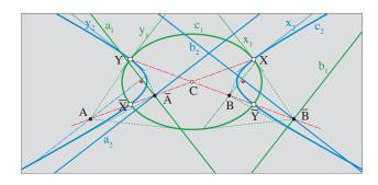
Figure 10: *The polar lines*  $a_1$  *and*  $a_2$  ( $b_1$  *and*  $b_2$ ) *are parallel to the tangent lines at* X (Y) *of conics*  $c_1$ *and*  $c_2$ , *respectively*.
