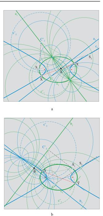
Figure 11: All central collineations with the green (blue) axis and a center on the blue (green) conic transform the green (blue) conic into green (blue) circles. The directions of the axes in figures a and b are conjugate to the common diametral chords of confocal conics. In both figures, the property that the tangent line at a center of collineation passes through the center of image circle is pointed out for the points  $S_1$  and  $S_2$ .
